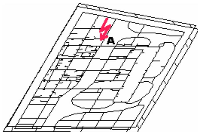
Figure 1. HV substation grounding grid – 3D view.
