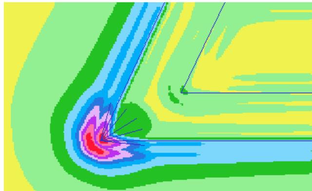
Configuration no. 18 - 3m long triple ground connexion added inside the substation-earthing corner.
