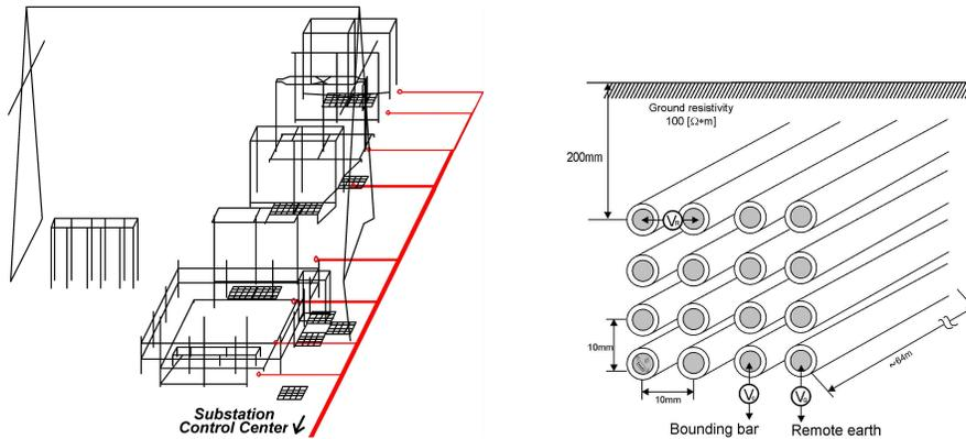
**Fig.2.** The part of substation model with control circuit wiring
