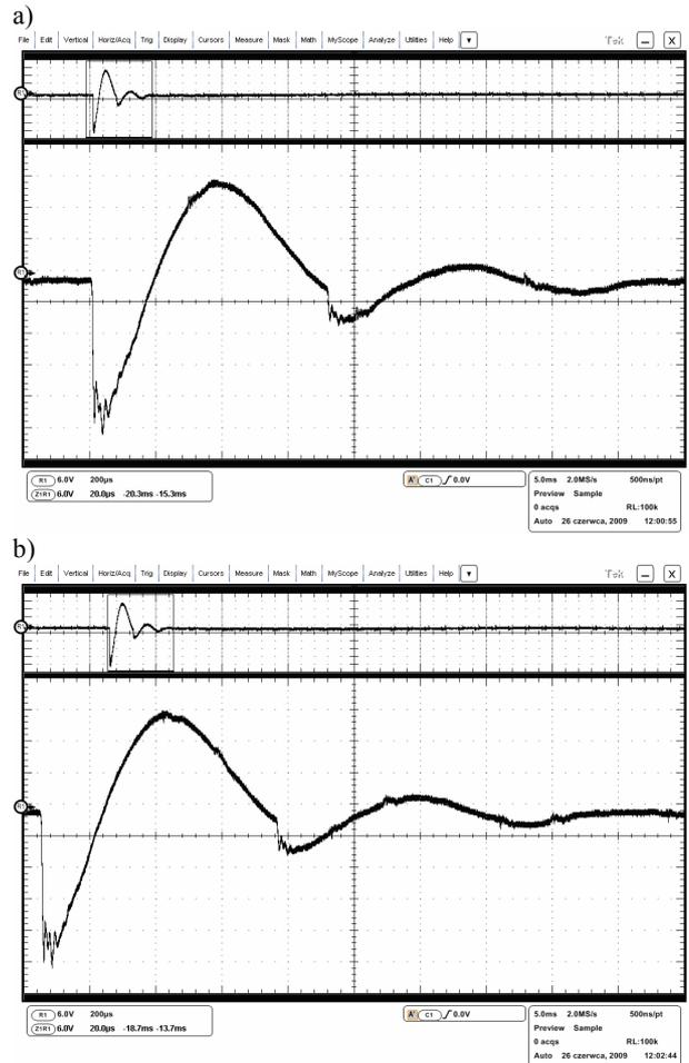
**Fig. 4.** Example waveforms of surge potentials with respect to remote ground recorded during the experiment at an earthing terminal inside a control cabinet on the 1-st floor
