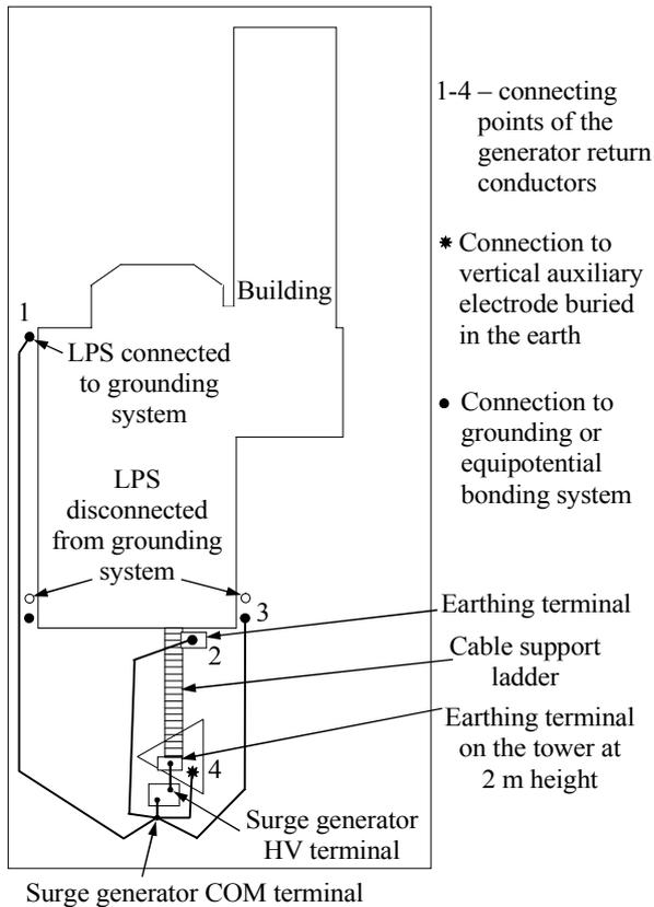
**Fig. 1.** Top plan of the telecommunication object together with the basic layout of the surge generator circuit
