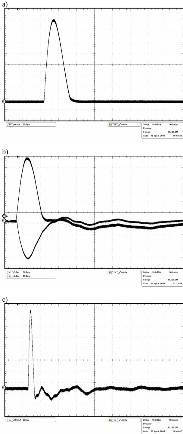
**Fig. 3.** Example waveforms of surge currents recorded during the experiment: a) the total surge current; b) in earthing conductors of antenna cables at the entry to the building; c) in earthing conductor of a control cabinet on the 1-st floor
