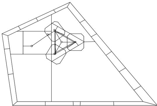
Fig. 2. GSM broadcasting station metallic structure in SESCAD (top view)
