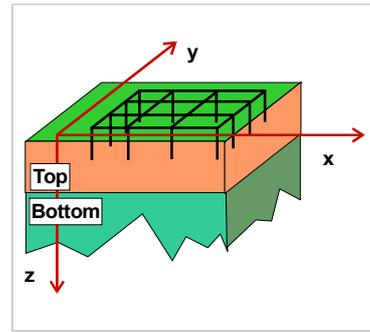
Fig. 7. Horizontal two layer soil type
