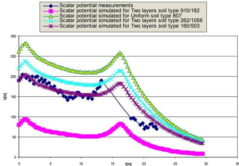
Fig. 9. Scalar potential compare between measurements and simulation
