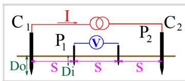
Fig. 3. Soil resistivity measurement. Wenner method
