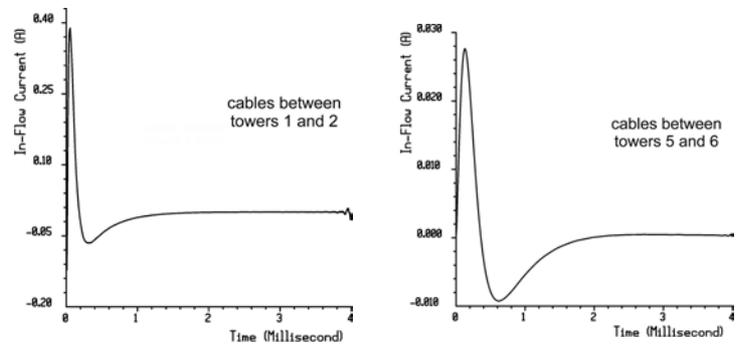
Fig. 7. Short circuit currents in telecommunication cables
