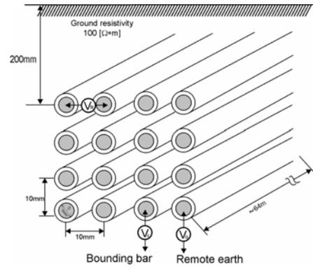
Fig. 3. Arrangement of cables under HV line
