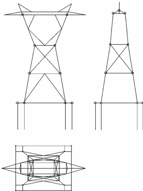
Fig.2. Model of HV tower with earthing system
