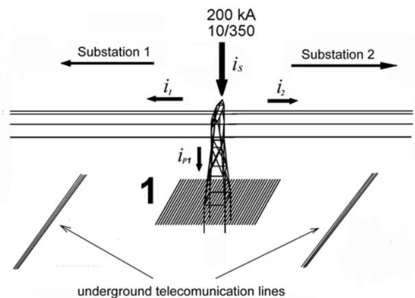
Fig. 4. Arrangement for the simulation of a direct lightning stroke to the top of the tower
