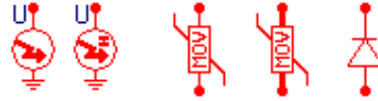
Fig. 2. Lightning voltage/current sources in ATP/EMTP program (from left side: two exponentials surge source, Heidler surge source, 1-phase metal oxide varistor, 3-phase metal oxide varistor, Zener's diode).
