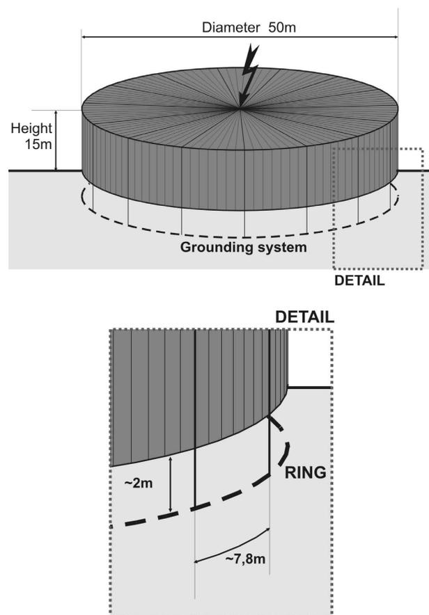
Fig. 1. Wire-grid approximation for the tank walls
