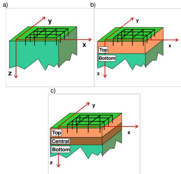
Figure 4 - Ground structure model – a) one layer one, b) two layers one, c) three layers one [4].
