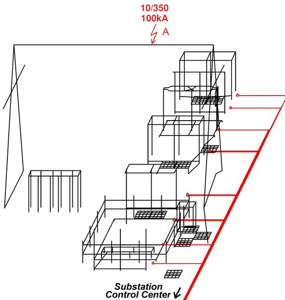
Figure 3 - HV substation line equipment field - 3D model
