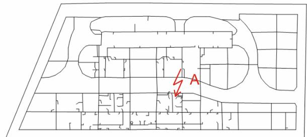
Figure 1 - Analyzed HV substation grounding grid – according the original documentation [2]
