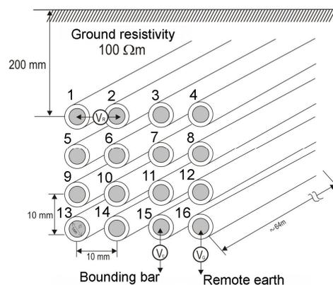
Figure 2 - Signal wires configurations in the telemechanics cable canal
