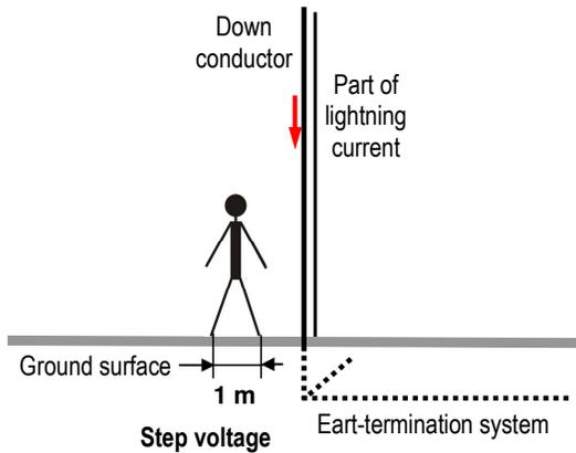
Fig. 2 - Transient step voltage.
