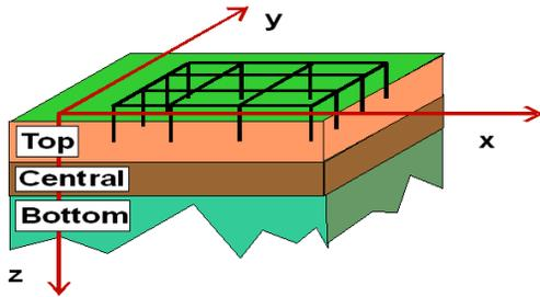
Fig. 10 - Soil structure with three layers top: 2mm - 2 Ω·m, central: 5 cm - 5 kΩ·m, bottom: 100 Ω·m.
