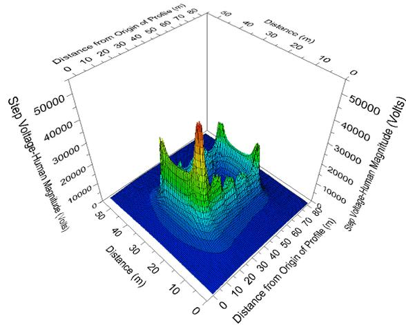
Fig. 11 - Step voltage distributions near building – additional semi-conducted top layer (lighting strike into the corner).
