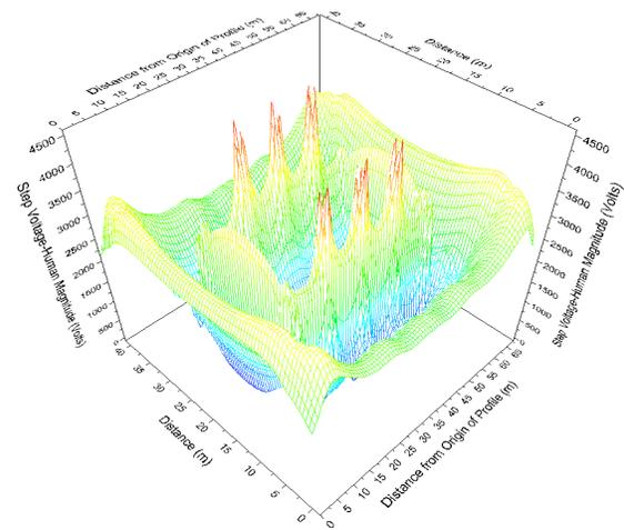
Fig. 7 - Step voltage distributions near building – uniform layer (lighting strike into the center).
