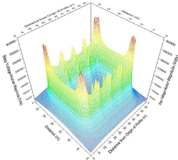
Fig. 6 - Step voltage distribution (maximal values) for one ring earth electrode.
