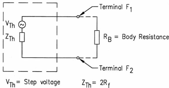
Fig. 3 - Step voltage circuit [8].
