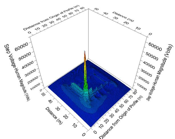
Fig. 8 - Step voltage distributions near building – two layers, top: 5 cm, 5 k $\Omega$ -m, bottom: 100  $\Omega$ -m. (lighting strike into the center).
