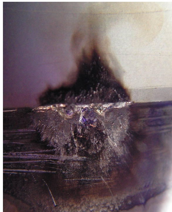
Fig. 7. 8/10 \mu s 55kA surge current result on the flagstaff interconnection point between sections
