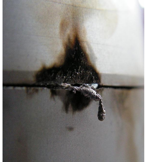
Fig. 6. 8/10 \mu s 55kA surge current result on the flagstaff interconnection point between sections
